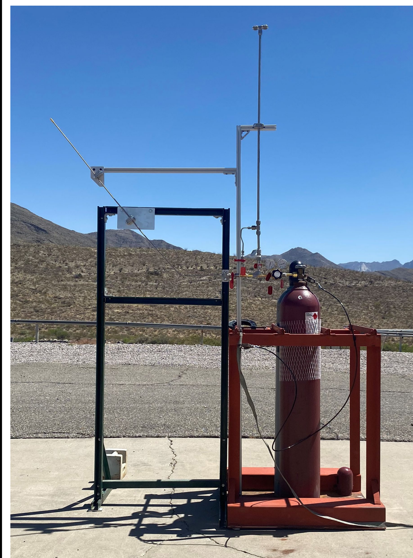
Figure 1: Hydrogen Flame Demonstration System
