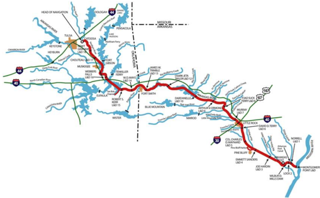
FIGURE 1. Map of the McClellan Kerr Arkansas River Navigation System (provided by the U.S. Army Corp of Engineers (USACE)). This map indicates all locks and dams in the system (outlined in red) with black lines across the river. State borders are indicated using dashed lines.
