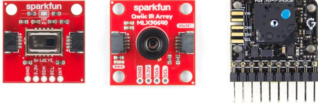
Image 2. All 3 thermal arrays - the Sparkfun AMG8833 (left), Sparkfun MLX90640 (middle), and FLIR Lepton mounted on the FLIR Pure Thermal Breakout (right), in order of increasing quality from left to right.
