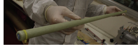
FIGURE 1: A Vacuum Bagging specimen before the bagging stage.
