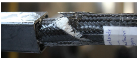
FIGURE 5: A damaged shaft at the end of torsion test.
