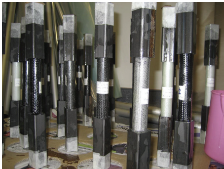
FIGURE 3: Shaft specimens with steel tube fitted to two ends.
