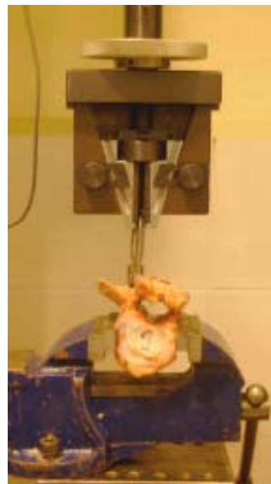
Figure 1. Pull out test with mechanical test device (Hounsfield H50KM)
